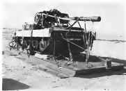
FIRST successful drop of an M56 gun on a stressed emergency platform. Destructive load has been compressed under load. Auto-tapping does extend beyond platform.
